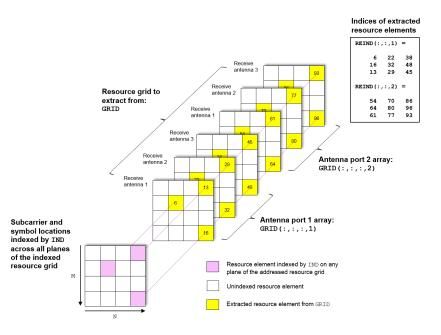
of *P M*-by-*N*-by-*NRxAnts* arrays, each associated with an antenna port. Resource elements are extracted from all planes within these arrays.
