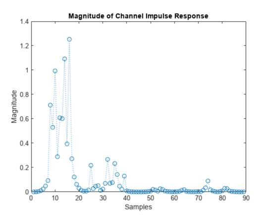
Estimate the timing offset by finding the peak of the impulse response magnitude.
